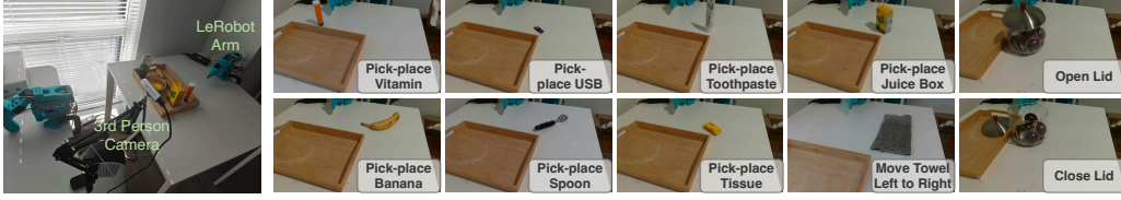
Figure 3: LeRobot experiment setup. We design 10 real-world tasks with different manipulation skills and objects with additional 2 unseen tasks for evaluating policy generalization.
