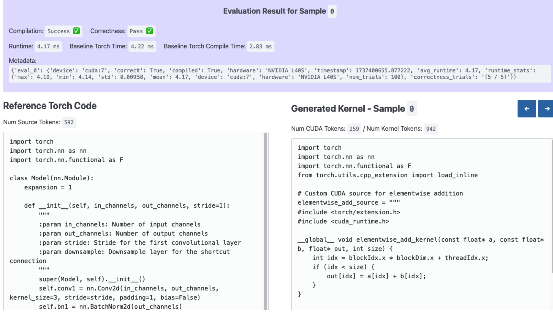
Figure 13. We provide a visual interface for kernel inspection. This allows us to easily examine kernel content, its performance, and compare across various techniques and configurations.
