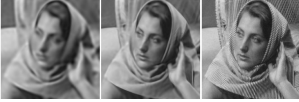
Figure 4: Smoothness control via SIREN’s frequency hyperparameter \omega . Overfitting SIREN to the right image with \omega = 30 (first) and \omega = 60 (middle) shows that smaller \omega leads to a smoother result.
