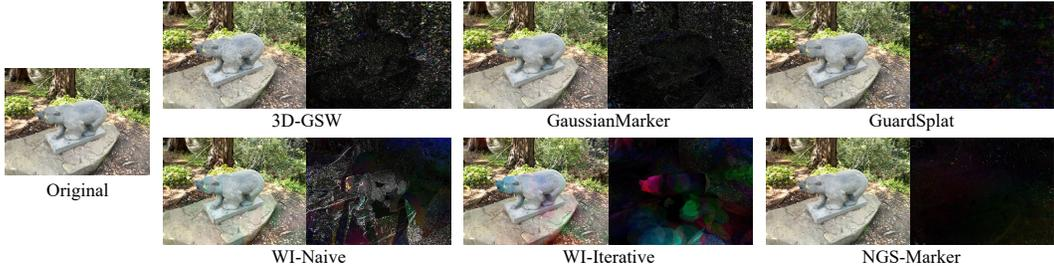
Figure 5: Visual comparisons in the bear scene with 16-bit watermark embedding. For better visualization, the difference images are amplified by a factor of 5. It can be seen that our method introduces negligible visual distortion.
