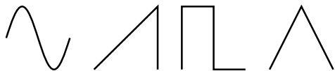
Figure 1: One period of each of the four toy waveforms: sine, sawtooth, square and triangle wave.
