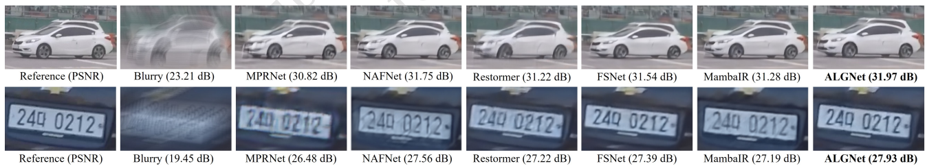
Figure 4: Image motion deblurring comparisons on the GoPro dataset [34]. Our ALGNet recovers perceptually faithful images.
