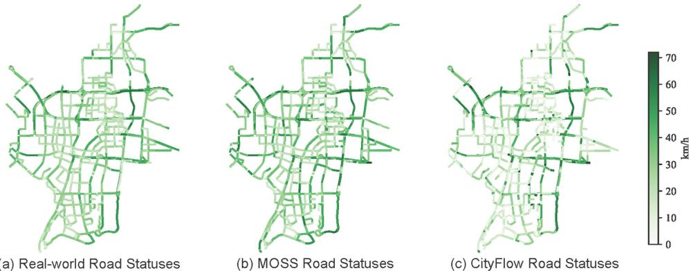
Figure A3: Visualization and comparison of road traffic status from (a) the Shenzhen dataset, (b) our proposed simulator, and (c) CityFlow. (best view in color)
