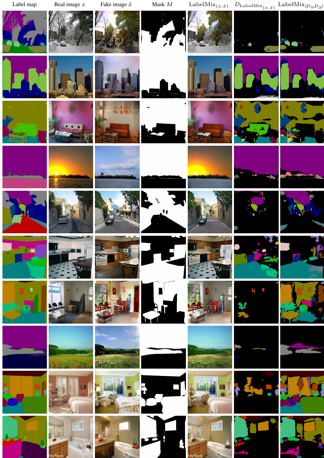
Figure L: Visual examples of LabelMix regularization. Real x and fake \hat{x} images are mixed using a binary mask M , sampled based on the label map, resulting in LabelMix _{(x,\hat{x})} . The consistency regularization then minimizes the distance between the logits of D_{\text{LabelMix}_{(x,\hat{x})}} and LabelMix _{(D_x,D_{\hat{x}})} . In this visualization, black corresponds to the fake class in the N+1 segmentation output.
