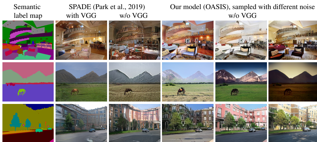
Figure 1: Existing semantic image synthesis models heavily rely on the VGG-based perceptual loss to improve the quality of generated images. In contrast, our model can synthesize diverse and high-quality images while only using an adversarial loss, without any external supervision.
