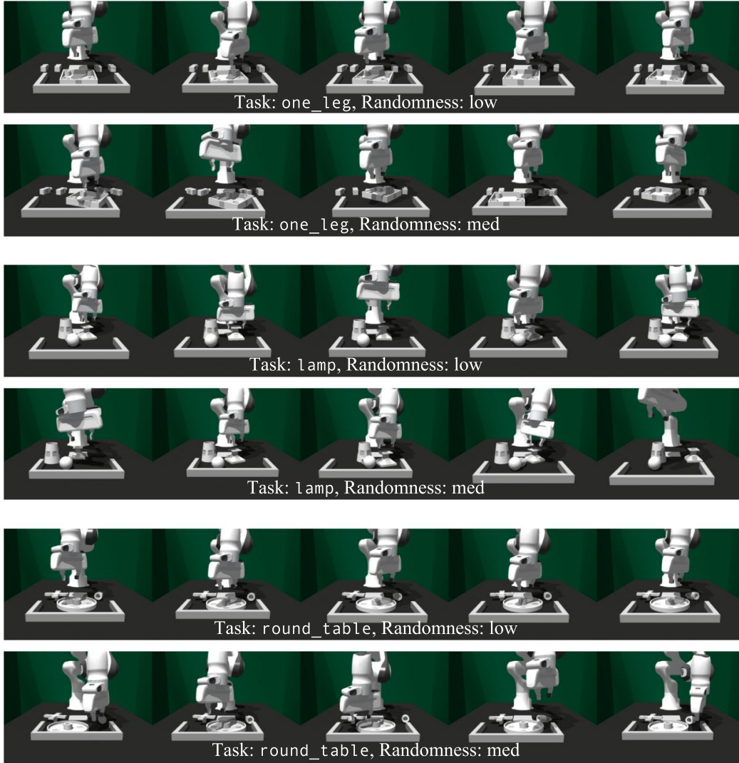
Figure 9: Examples of initial scene layouts for one_leg , lamp , and round_table with different levels of initial part pose and obstacle fixture randomness
