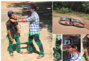
Stabbing pose. Singh's deep learning network uses 14 key points on the human body to identify violent poses such as strangling, punching, kicking, shooting, and stabbing. Courtesy S.N. Omkar.
