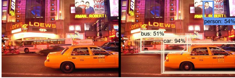
Figure 1: Examples of bounding box uncertainties on the object detection task. The thicker boundary represents the original model prediction, and the thinner lines represent ten quantiles (between 0.1 and 0.9) predicted via QFR. High-confidence boundaries (such as those of the car) are closer together, while low-confidence boundaries (e.g., the bus which is blurred and partially occluded) are asymmetrically spread out, reflecting the advantages of non-Gaussian uncertainty estimation.
