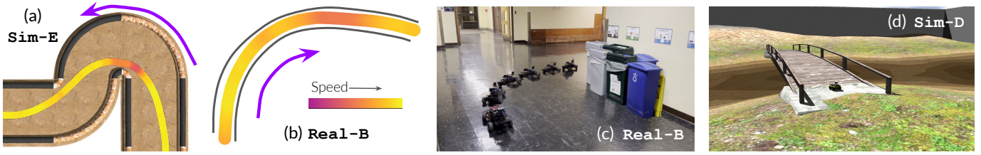
Fig. 2: Emergent behaviors with FastRLAP. (a, b) show the robot’s telemetry data in environments Sim-E and Real-B after 30 minutes of autonomous practicing. We find that directly minimizing lap times with RL results in the emergent discovery of a “racing line”, braking as late as possible to maintain speed in and out of tight corners (a, b) and drifting on slick surfaces (c). In a challenging outdoor environment Sim-D , the robot infers that the bridge is faster than driving through mud via visual correlation, learning a fast driving policy (d). All the above graphics are rendered using telemetry from our real-world (b, c) and simulated (a, d) experiments. The third-person views are provided for visualization only, and are not available to our system. Please see supplemental material for videos of these emergent behaviors.
