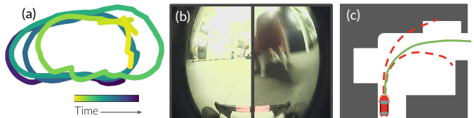
Fig. 4: High-speed visual navigation faces challenges due to sensing, perception, and dynamics: (a) noisy odometry and localization errors across multiple laps, (b) overexposure and motion blur in the visual observations, and (c) over-/under-steer due to complex dynamics.
