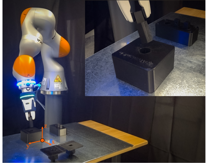
Fig. 1: Peg-in-hole assembly with the KUKA LBR iiwa.
