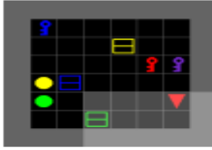
Figure 4. An illustration of one BabyAI task, PutNextLocal: "put the blue key next to the green ball". The shadow area represents the observable space of the agent.
