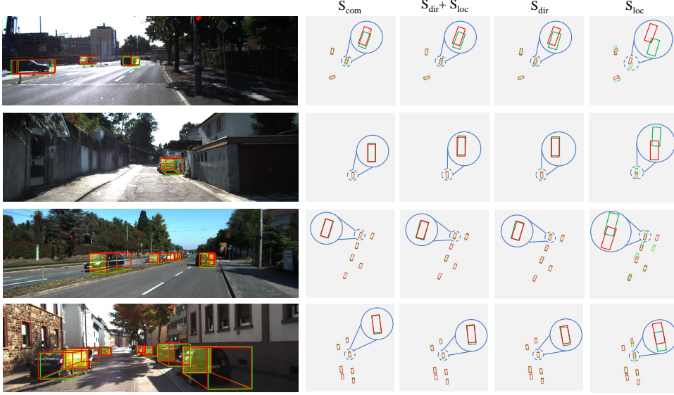
Figure 4: Qualitative examples on the KITTI validation set. Each row displays a 3D scene detection result along with four BEV visualizations. The BEV visualizations reflect the differences in depth. From left to right: S_{com} , S_{loc} + S_{dir} , S_{loc} , S_{dir} . Red represents the GT of the box and green represents the prediction box.
