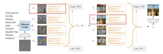
Figure 1: **Dynamic CFG**. We propose to perform a greedy search over multiple CFG scales and select the one that maximizes the latent evaluators' scores at each sampling step. The evaluators are small-scale and operate directly in the diffusion latent space increasing the computational overhead during inference by only 1%. Finally, for combining scores by multiple evaluators, we propose an adaptive weighting dependent on the denoising timestep.
