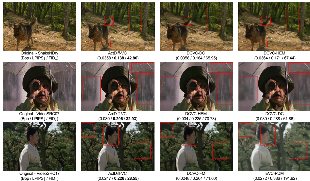
Figure A2: Additional qualitative comparison examples extending Figure 5 on representative sequences from the UVG dataset (ShakeNDry) and the MCL-JCV dataset (videoSRC07 and videoSRC17). For each example, we compare ActDiff-VC with competing methods at similar or higher bit rates. The numbers below each reconstruction report per-video BPP, LPIPS, and FID (lower is better). Red boxes highlight regions where competing methods exhibit stronger artifacts, blur, or structural degradation, while ActDiff-VC better preserves visually plausible textures and object boundaries.
