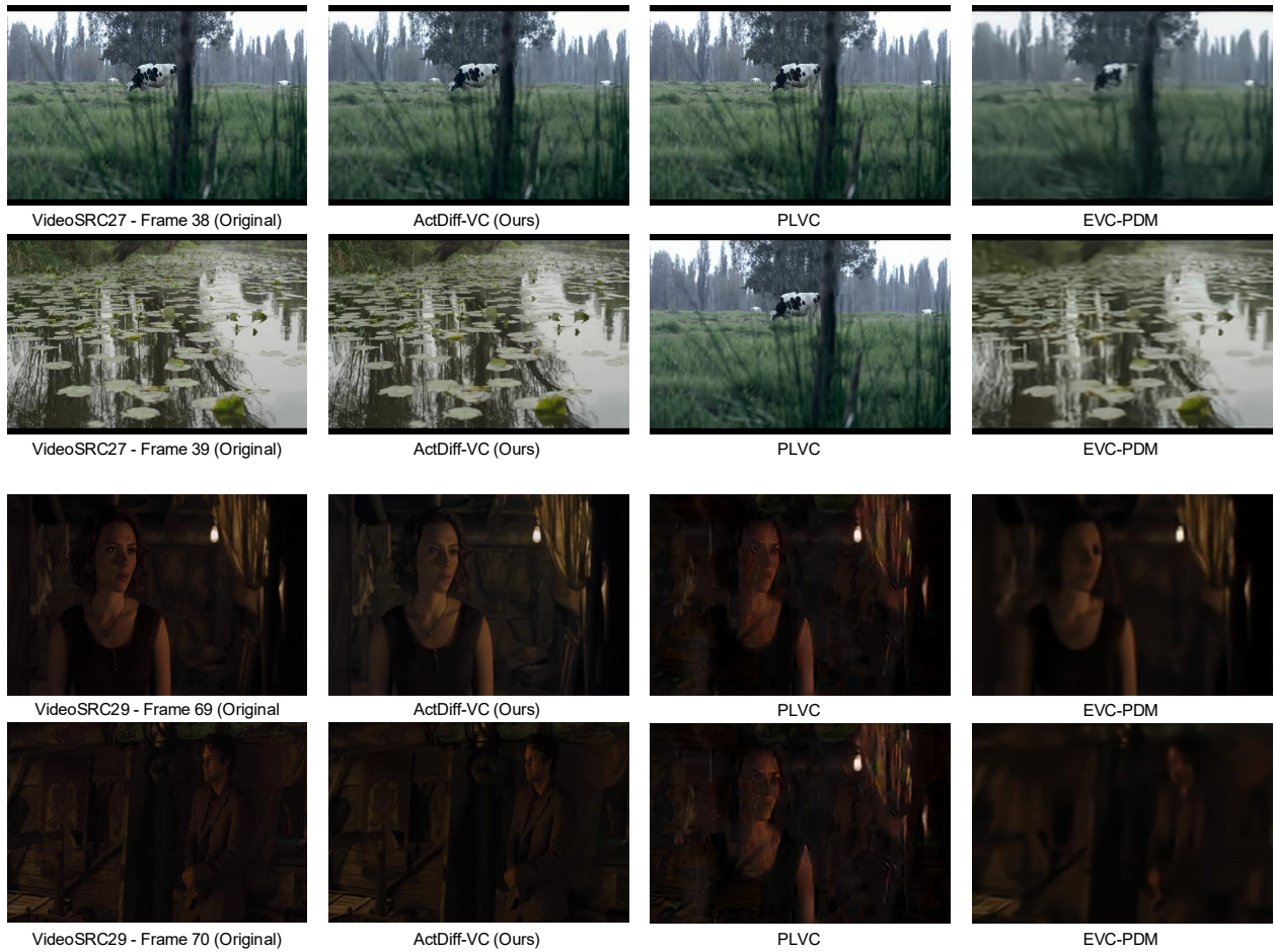
Figure A4: Additional visualizations of the proposed content-adaptive keyframe selection mechanism on MCL-JCV sequences videoSRC27 and videoSRC29. Similar to the examples in Figure 6, ActDiff-VC successfully adapts to abrupt scene changes by selecting new keyframes when needed, leading to higher-quality reconstructions after scene cuts. In contrast, PLVC often fails under its fixed key-frame schedule, while EVC-PDM requires substantially higher encoder-side computation and still produces weaker visual quality.
