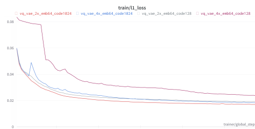
Figure 5: Plot of reconstruction loss when training VQ-VAE with different codebook sizes and downsample factors. With small codebook size ( |V| = 128 and s = 4 ), reconstruction error is significantly higher than model trained larger codebook size ( |V| = 1024 ).
