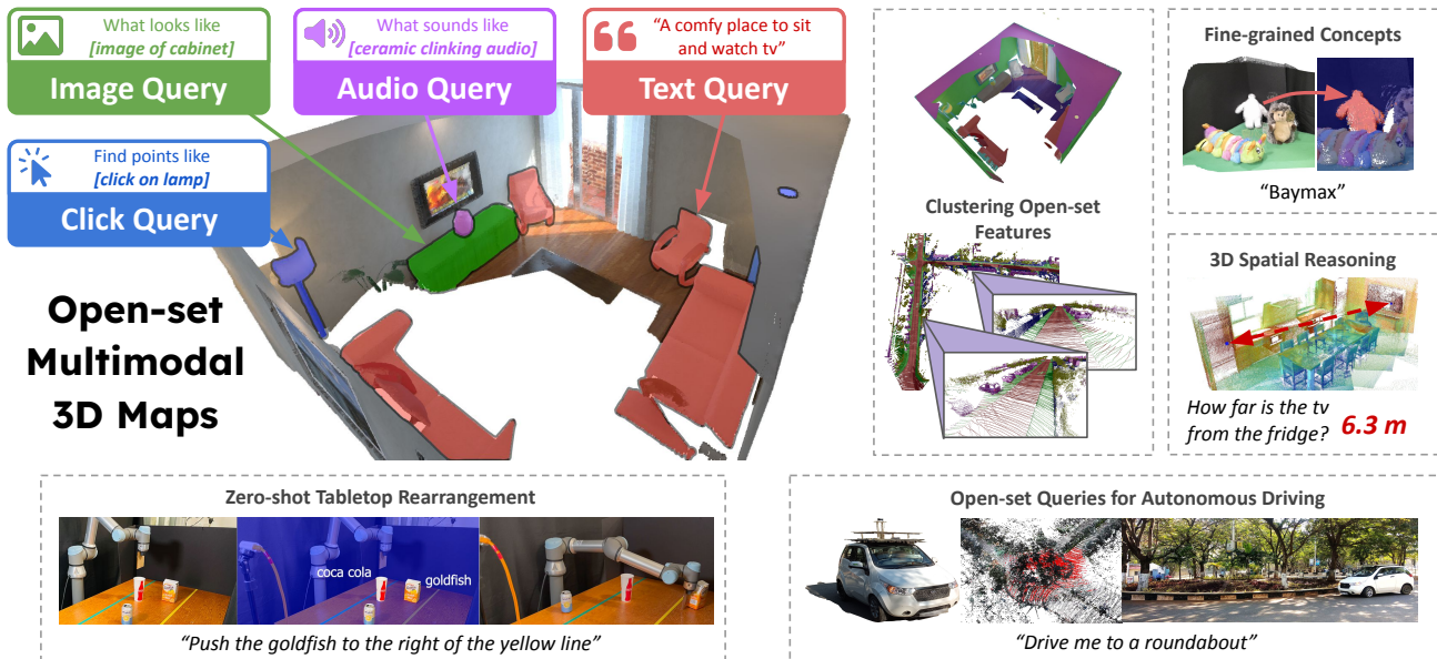
Figure 1: ConceptFusion is a real-time approach to building open-set multimodal 3D maps from RGB-D images, and features from foundation models like CLIP and DINO. These maps, built on-the-fly, can be queried for arbitrary concepts specified as text, images, audio samples, or clicks on the 3D map. The fused features implicitly capture semantic concepts, as evident by visualizing clusters obtained from a K-means algorithm. ConceptFusion features are significantly more adept at retaining fine-grained concepts, such as the disney character “Baymax”. We also build 3D spatial reasoning modules that enable reasoning about frequently observed spatial relationships. We demonstrate the applicability of ConceptFusion to the real-world robotic tasks of tabletop manipulation of novel objects, and an urban autonomous driving setting. (Webpage)
