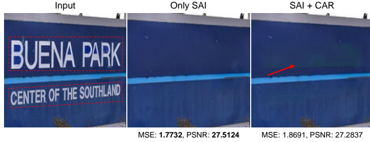
Figure 23: Adding CAR when SAI alone is sufficient tends to introduce color shifting artifacts, which in turn degrades performance in terms of MSE and PSNR.
