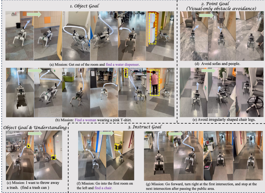
Figure 4: Real-world deployment. It shows third-person view of the three different navigation tasks which are deployed in a zero-shot setting. The gradient blue arrows indicate the trajectory, and the yellow box marks the target location. Our model demonstrates highly effective navigation performance on the real quadruped robot.
