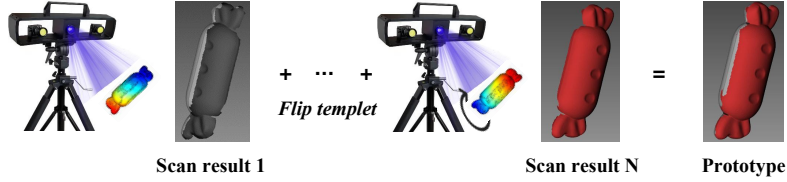
Figure 3: A prototype in the training set is made from two or more scan results.
