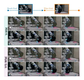
Figure 15: Wipe Cloth task. V-WM rollouts show artifacts and miss contact, leading to ineffective wiping, while VT-WM maintains contact and produces consistent cloth displacement in execution.
