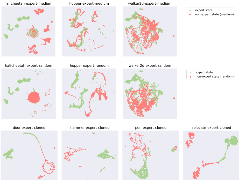
Figure 9: We use UMAP to reduce the dimensionality of states in different D4RL tasks. Expert states are visited by expert behavior policies, and non-expert states are from the medium, random or the cloned policies. We enlarge the dot size of expert states for clarity.
