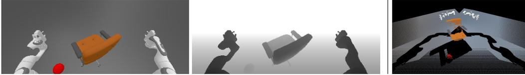
Figure 4: RGB-D (RGB/Depth) and point cloud observations in ManiSkill. Left two images: RGB-D image from *one* of the three cameras mounted on the robot. The three cameras together provide an ego-centric panoramic view. Right image: visualization of fused point cloud from *all* three cameras. The center of robot body cannot be seen since the captured point cloud comes from an ego-centric view. Parts of the chair are occluded by itself (as cameras are mounted on the robot).
