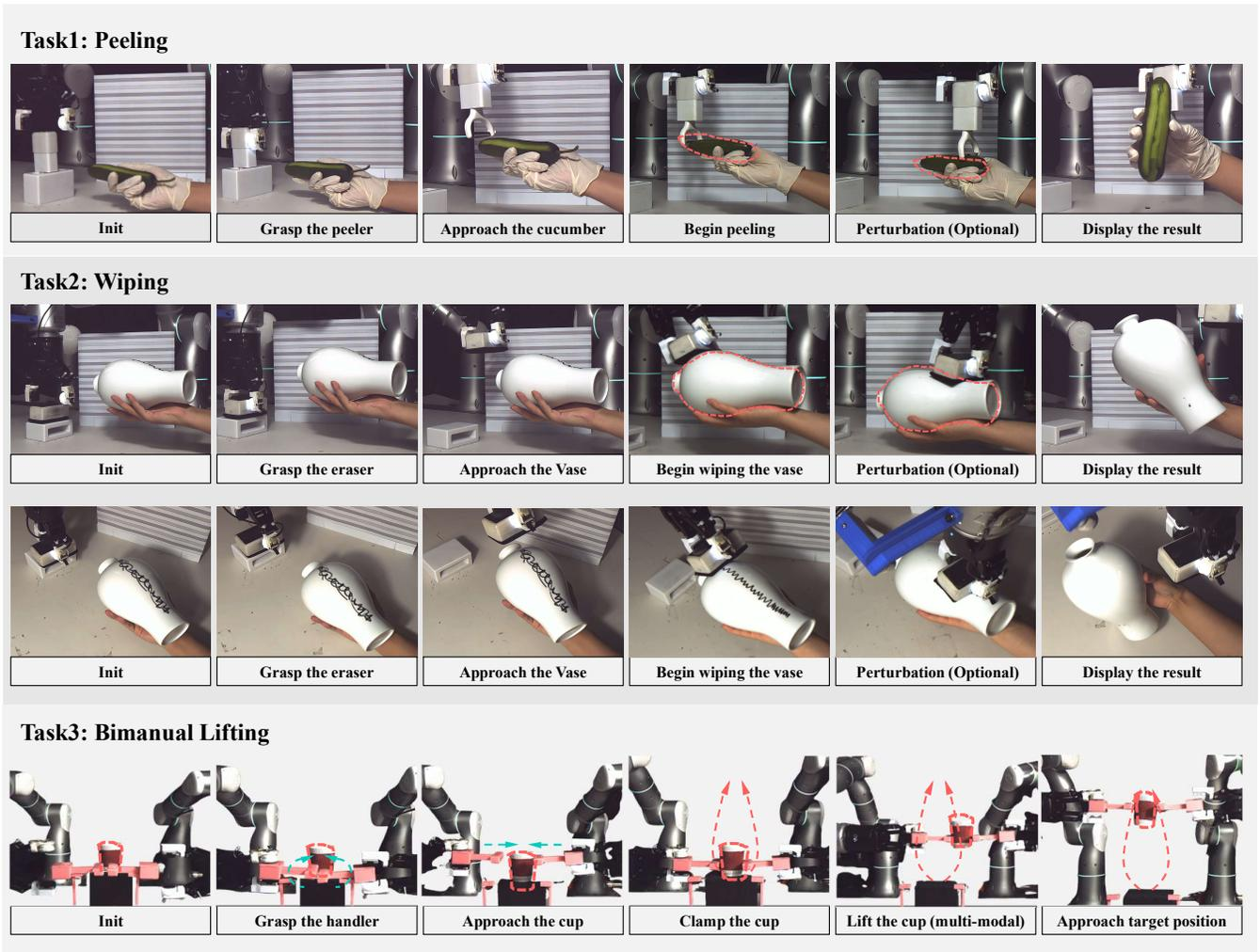
Fig. 11: Three experiment tasks including *Peeling*, *Wiping* and *Bimanual Lifting*.
