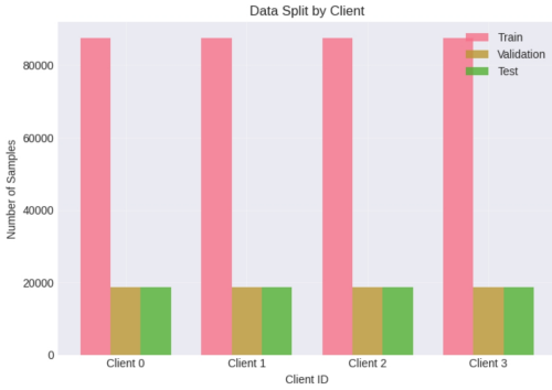
Figure 4: Schematic illustration of the period-based dataset partitioning strategy used to construct federated clients. The full dataset is sorted by grating period and divided into four equal-sized, non-overlapping client subsets, each subsequently split into training (70%), validation (15%), and test (15%) sets.
