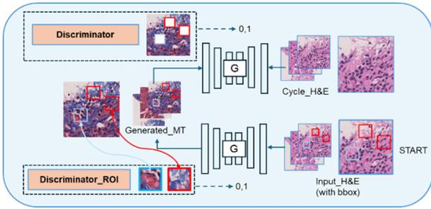
Fig. 2: H&E tiles are processed through a generator to generate MT-stained tiles, with discriminators trained on labeled fibrosis/non-fibrosis regions refining the output; cycle consistency loss ensures fidelity between original H&E and regenerated tiles.
