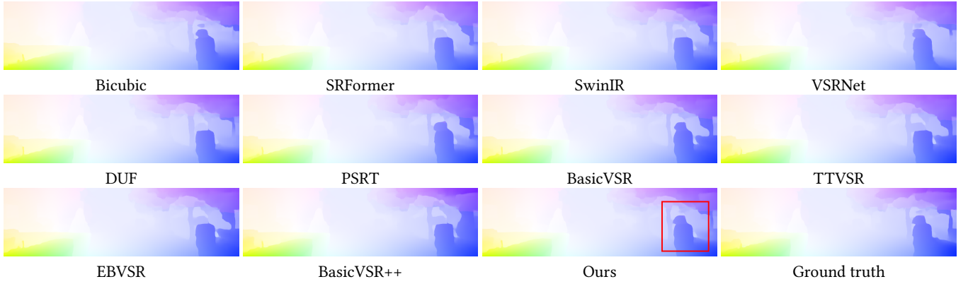
Figure 5: Temporal consistency comparison on the 4× asymmetric event-guided VSR task. We show the estimated optical flow of the results from different methods using the pre-trained RAFT [56].
