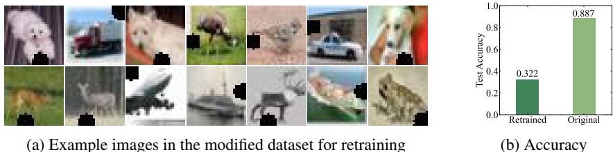
Figure 1: Retraining on the modified dataset. Our malicious modification scheme perturbs a small fraction of background pixels but introduces a high correlation with classes. The test accuracy on the unperturbed test set shows that the retrained model ignores the remaining features but learns to mostly rely on introduced artifacts for classification. Hence, the low test accuracy here is not due to information removal, but due to not learning from the true class-related information.
