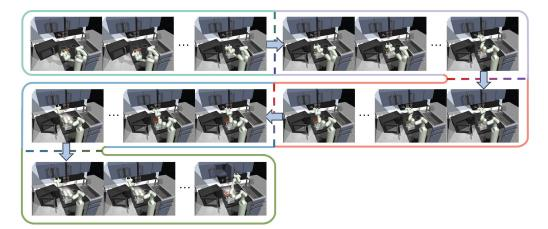
Figure 7: Skill extraction results using VanTA in kitchen-mixed: sequentially 1) open the microwave, 2) red flame circles appear on stove as it turns on the gas stove, 3) rotate the knob to turn on the white light above the stove, which is the left one among those knobs, and 4) open the cabinet.
