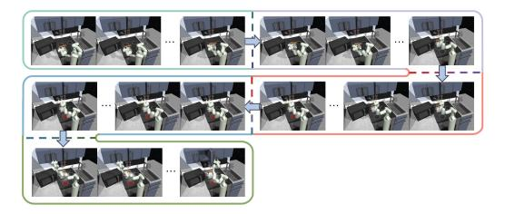
Figure 9: Skill extraction results using VanTA in kitchen-partial: sequentially 1) Move the kettle, 2) red flame circles appear on the stove as it turns on the gas stove, 3) rotate the knob to turn on the white light above the stove, which is the left one among those knobs, and 4) open the cabinet.
