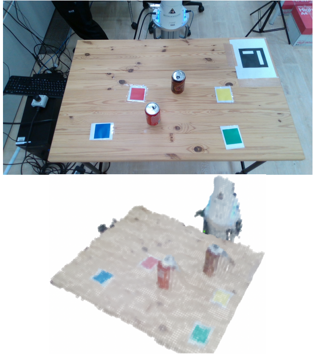
Fig. 1: 720 \times 1280 image view from the RGBD camera (top) vs. 100^3 voxel view (bottom). Fine-grained semantic information somewhat diminished in the voxel view.
