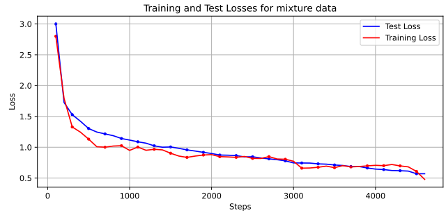
Figure 4: Fine-tuning performance on a larger mixed dataset with mixing ratio \alpha = 0.5 . The training and test loss curves on the held-out domain-specific dataset exhibit desirable convergence, with the test loss closely following the training loss, contrasting the overfitting observed when fine-tuning on single datasets. The results suggest that increasing the overall training data size while maintaining an optimal mixing ratio can amplify the regularization effect of dataset mixing.
