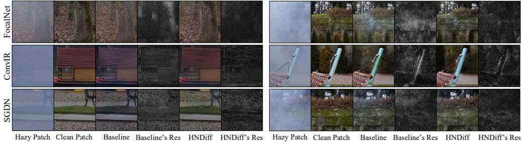
Figure 4: Qualitative results on the O-HAZE (left) and NH-HAZE (right) datasets. “Res” denotes residual maps between outputs and ground truth, where darker intensities indicate smaller errors.
