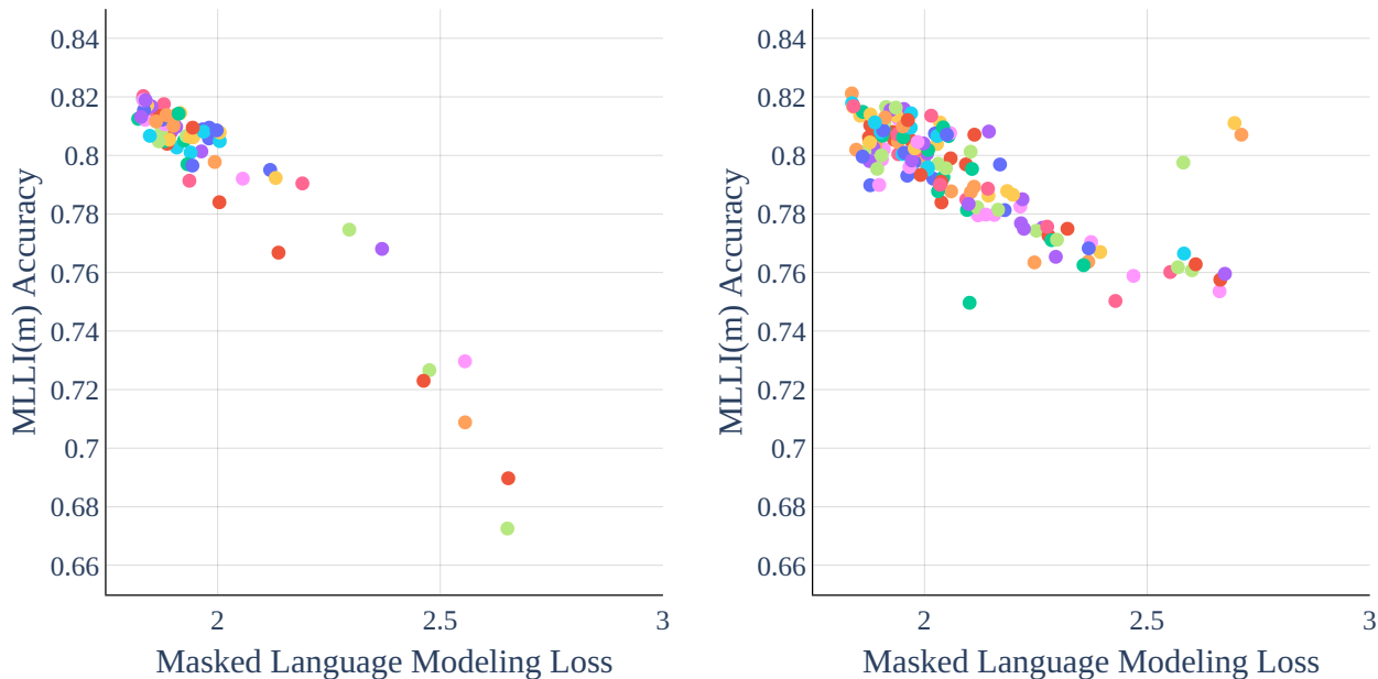
Figure 5. Relationship between pretraining loss and downstream performance. Left: for all architecture variations considered (see Table 9 for details). Right: for all training variations considered (see Table 12 for details).
