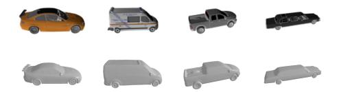
Figure 22: **Single-view reconstruction.** Given a single RGB image (top), a lightweight ResNet-18 encoder predicts part latents and poses for our pretrained part decoder, which reconstructs the composite 3D shape (bottom). The model recovers coherent part layouts and overall geometry.
