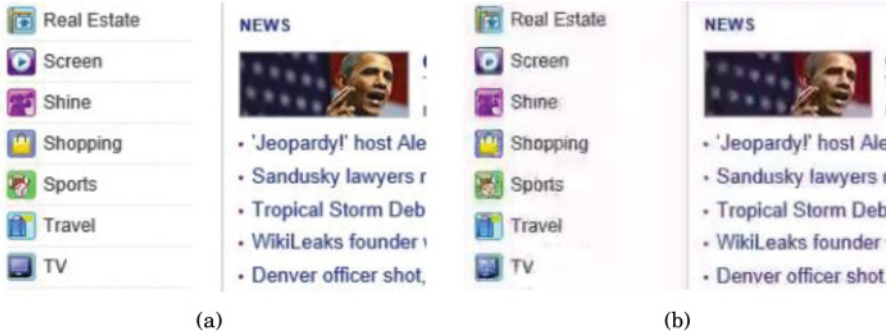
Fig. 14. Visual quality comparison between the proposed layered coding scheme and x264. (a) Reconstructed from the proposed scheme (bitrate: 1.83Mbps). (b) Reconstructed from x264 (bitrate: 1.84Mbps).
