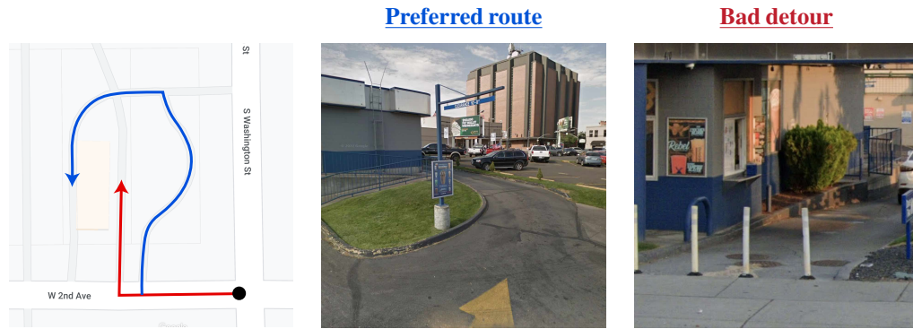
(a) Spokane A road is incorrectly marked as drivable. The correct route takes users through the designated drive-through, as desired. The sparse model learns to correct the data error with a large negative reward on the flex-posts segment.
