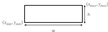
Figure 5: Illustration of layout as a bounding box associated with each word in the text input sequence.
