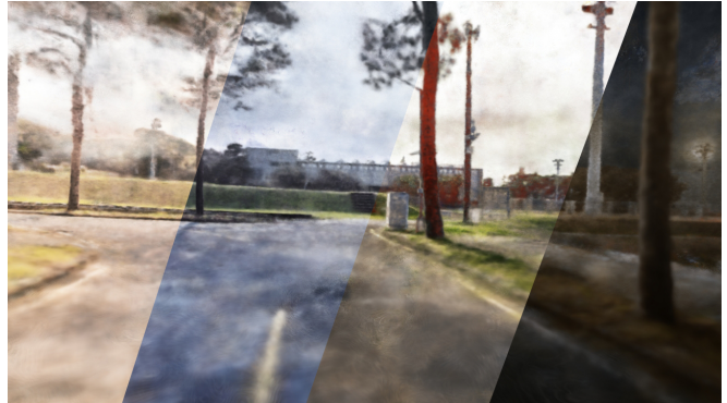
Fig. 1: Visualization of the scenes rendered by DriveEnv-NeRF for emulating diverse lighting conditions using different setups of the appearance embedding for training policies.
