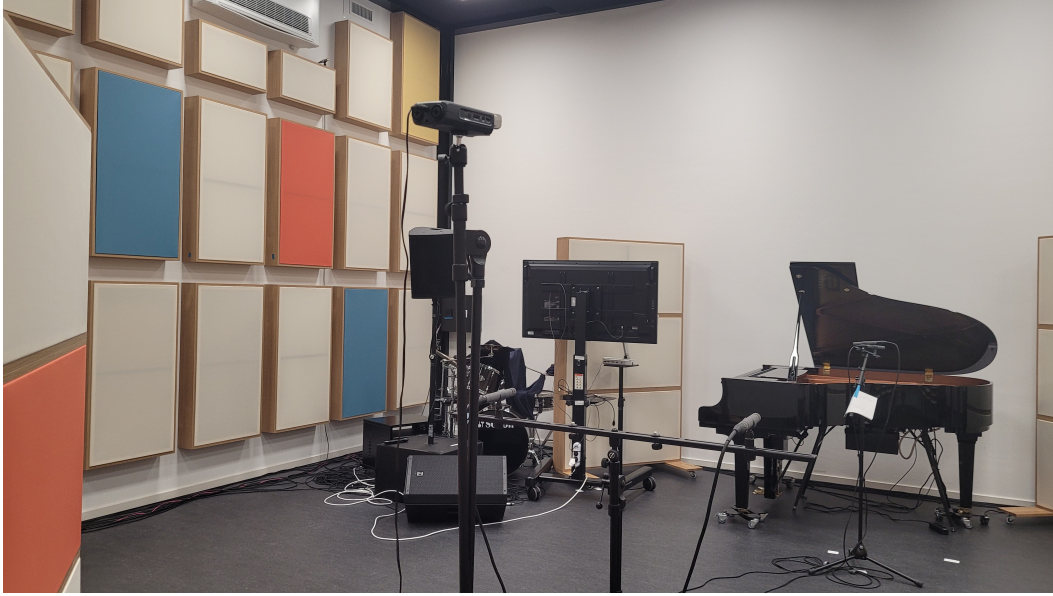
Figure 5: MIDI-controllable reproduction piano (Yamaha C3X Enspire Pro) in the acoustically optimized studio with different microphone setups. Handheld recorder, AB-microphones for room sound and ORTF microphones for close-miking.
