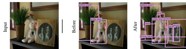
(a) Optimize mAP: 39 → 54, results in a much higher recall and learns box prediction confidences.
