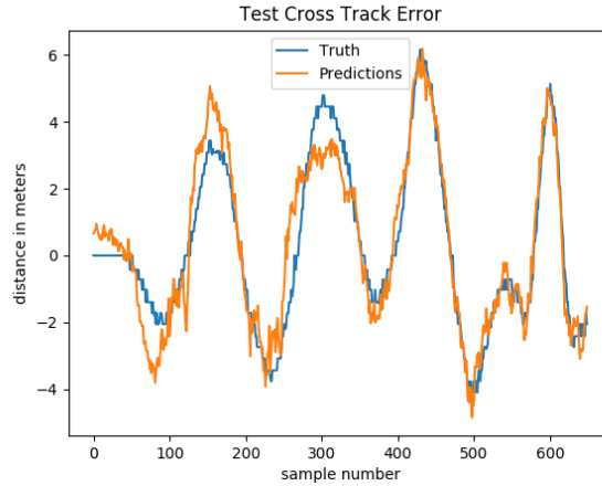
Figure 2: Preliminary test results for estimating the cross track error using MobileNetV2 in the X-TaxiNet architecture. The test data included images collected while taxiing on a different set of taxiways than during training.
