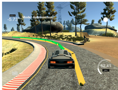
Figure 2: MCTS braking in front of a sharp turn in Udacity Simulator. MPC never shows braking behavior in the experiment.
