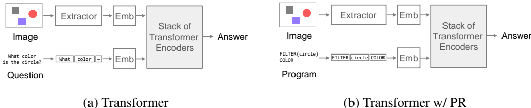
Figure 3: Transformer-based Baseline Methods . (a) Standard Transformer (Transformer) takes an image and a question as inputs. (b) Standard Transformer with programs (Transformer w/ PR) takes a program as an input instead of the question. Emb denotes visual/word embeddings. These approaches use the same visual inputs and Transformer encoder structure.
