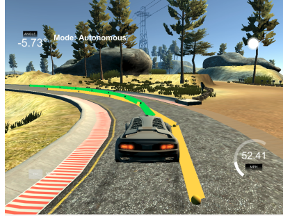
Figure 2: MCTS braking in front of a sharp turn. MPC never shows braking behavior in the experiment.
