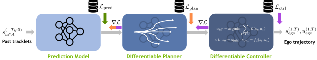
Figure 2: DiffStack is comprised of differentiable modules for prediction, planning, and control. Importantly, this means that gradients can propagate backwards all the way from the final planning objective, allowing upstream predictions to be optimized with respect to downstream decision making.
