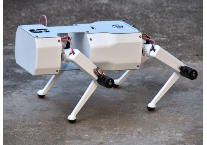
Fig. 1. Pupper Robot : a low-cost, agile quadruped designed for teaching an AI/Robotic curriculum and for studying novel reinforcement learning techniques
